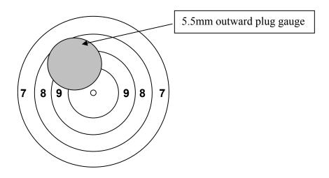
In the diagram below the outward scoring plug gauge shows the outside edge of the flange lying within the 8 ring, therefore the shot is scored as a 10.
