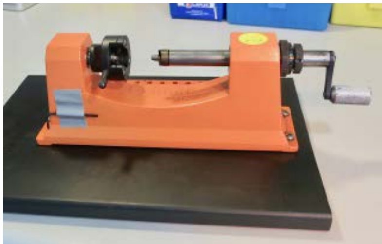
Lyman case length trimmer set to the magic case length of 1.555" for 6BR.
