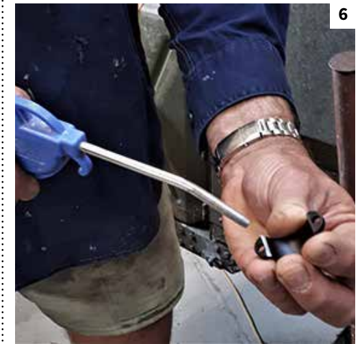
Step 6: Blow dry after neutralising with water.
