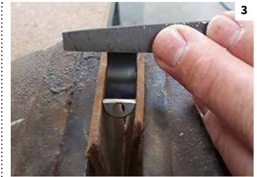
Step 3: File the sharp edge.
