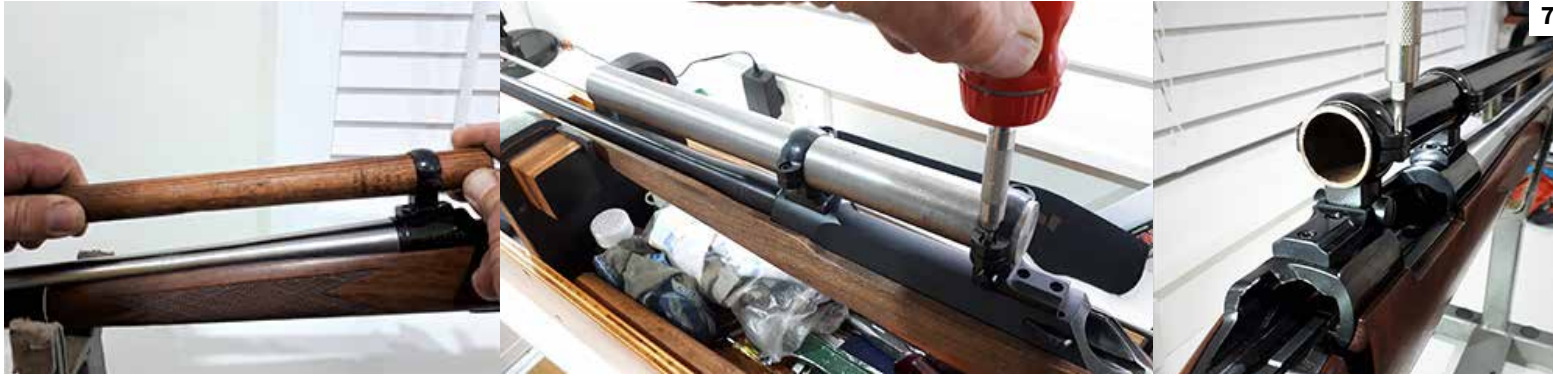
Step 7a: Timber dowel; Step 7b: Steel bar stock; Step 7c: Heavy wall steel pipe as an alternative to solid bar stock.
