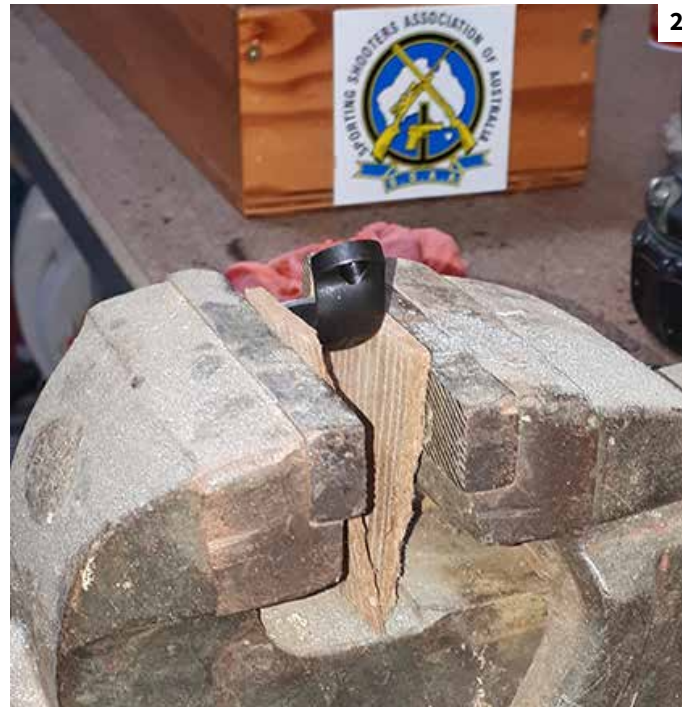
Step 2: Place rings in the vice between soft jaws.
