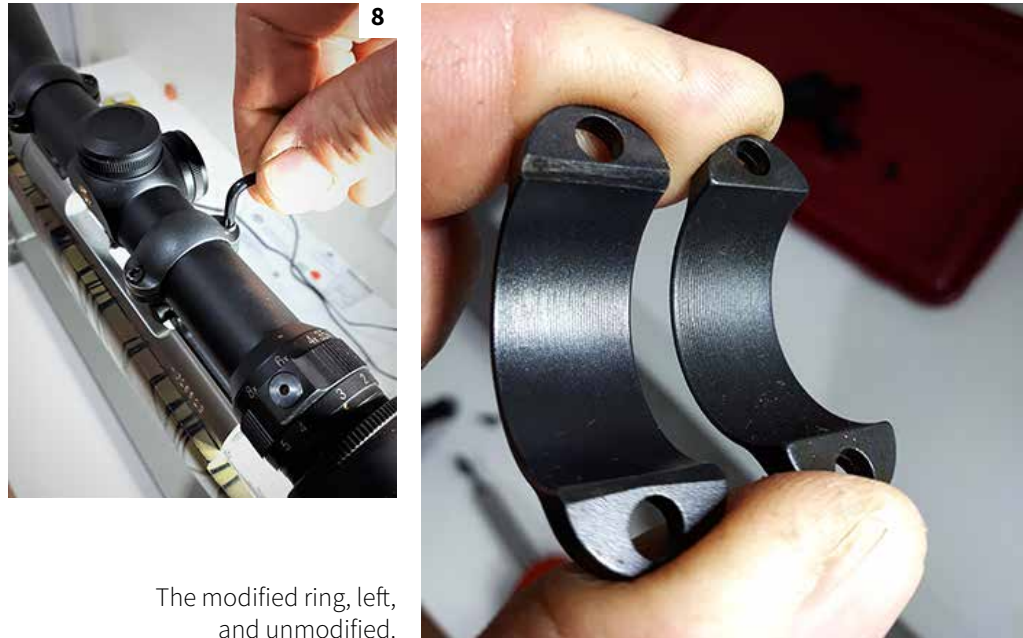
Step 8: Tighten the screws with Torx tool provided.
