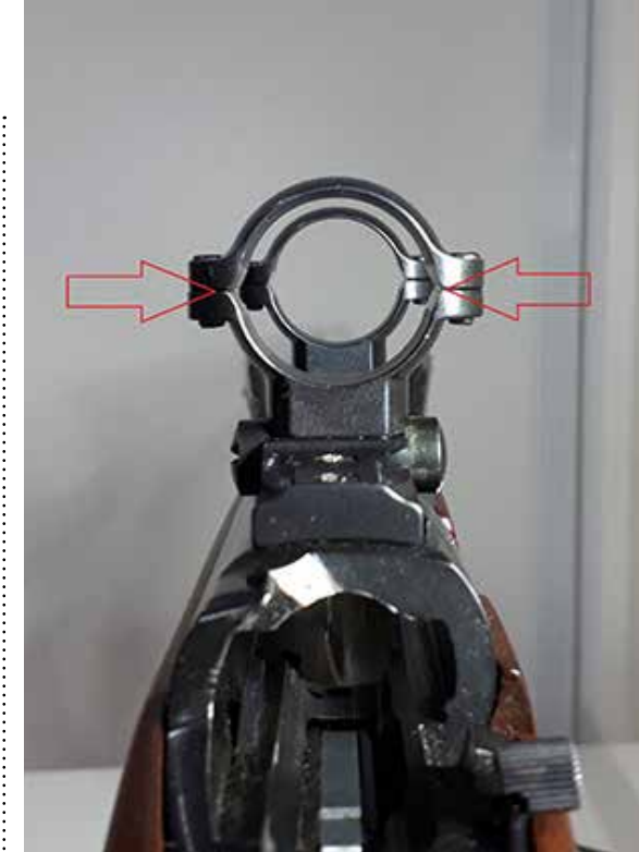
Red arrows indicate slight modification to the rings.
