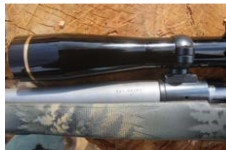
The essential 1:8" twist Tobler Stainless steel barrel makes the concept of longer calibre bullets viable.
