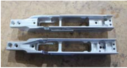
Differences may be subtle but important in the chassis inlet between models - Tikka T3 inlet (top) and Howa 1500.
