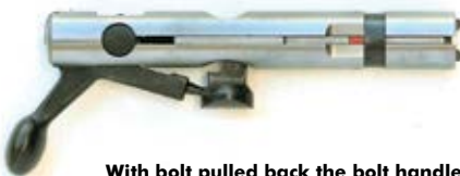
With bolt pulled back the bolt handle pivots on the blue pin at the back of the body, drawing the locking bolt out and allowing the action to be opened.
