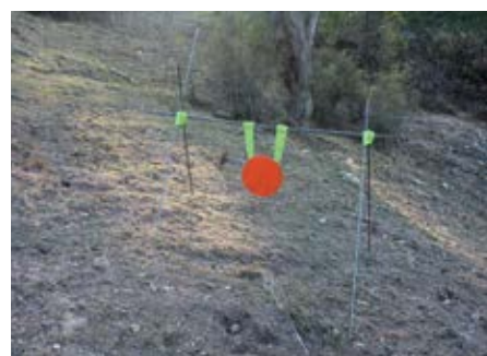
The kit can be set up on sloping ground by adjusting the length and angle of the rebar legs.
