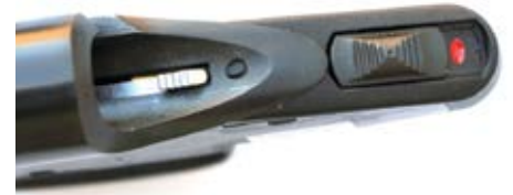
Rear of receiver showing serrated steel bolt stop that must be depressed to remove the bolt from the receiver. The sliding safety catch must also be engaged.
