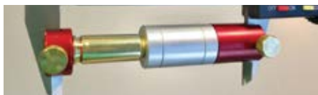
Headspace bushing and anvil. The reference plane is about middle of the shoulder and measurement is a reference number to set up the body die to 'bump' the shoulders back after repeated firings stretches the brass.
