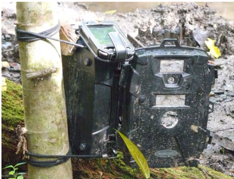
Plate 29 Motion sensing camera positioned in the field with handheld PDA uploading data. [2009]
