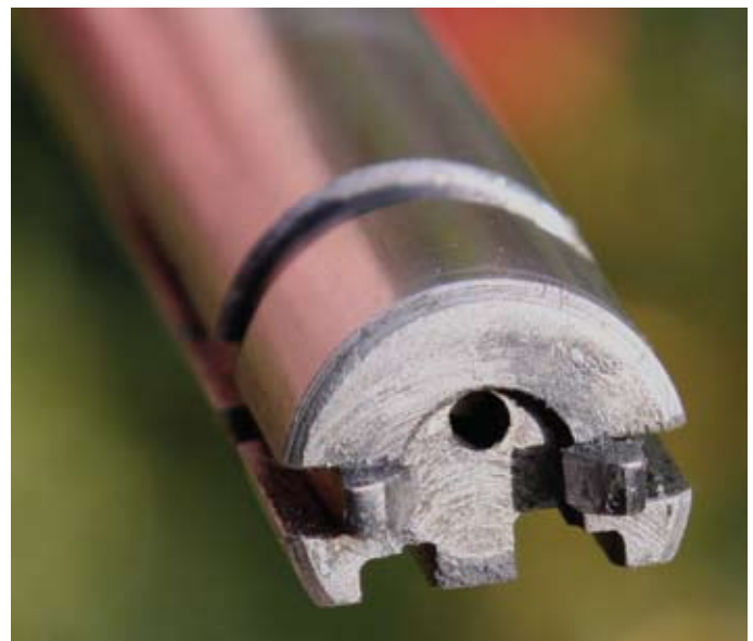
This rimfire rifle bolt shows grime and blowback after firing only 60 rounds. It can easily be cleaned up with a toothbrush.
